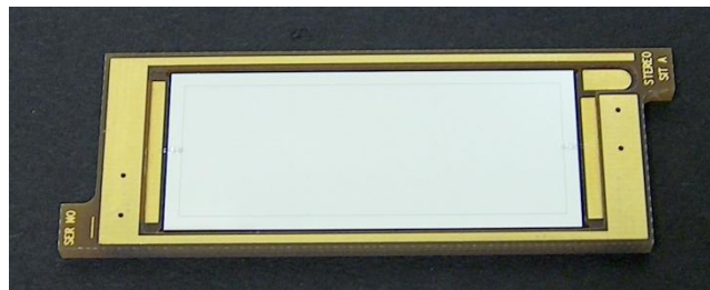
MSX 060 2M/2M mounted on a double recessed FR4 transmission package.
