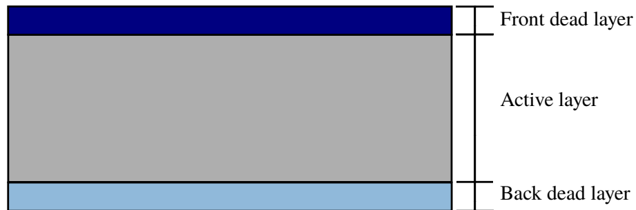
Figure 2.1: The sketch depicts the simple layout of the pad detector. Note, that this is only a sketch and thus does not have any scaling ratio. You should thus be aware that the sizes at the two axes are skewed.
