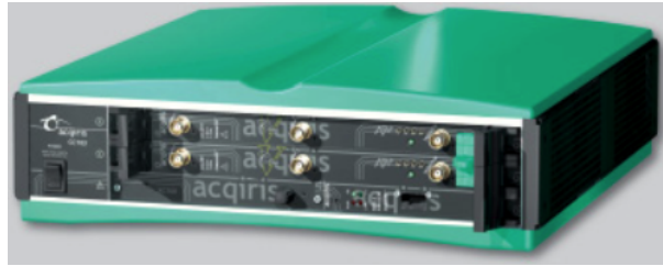
Figure 6.7: Picture of the Acquiris digitizer crate with 440DC cards. From [77].
